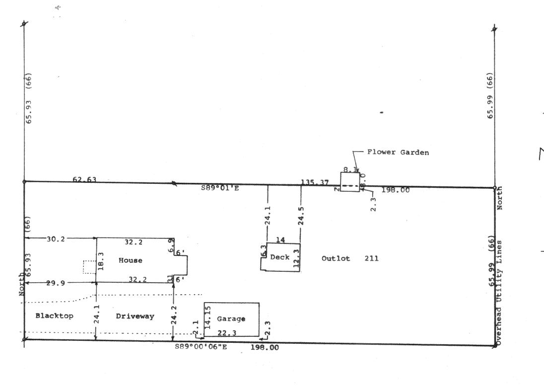
Scale - 1" = 20" $\emptyset = 3/4$ " Iron Pipe Found ∀ = ⅓ X 24" Iron Pipe Set o = 1" X 24" Iron Pipe Set (0.00) = recorded distance Bearings referenced to the assumed bearing of North along the east line of Wood Street Survey ordered by: Churchill Real Estate 322 Park Street Walworth, WI 53184
